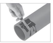
**Step 6:** Using an appropriate applicator, that corresponds to half the pipe diameter, apply Primer inside the connection bag till the surface is malleable.
